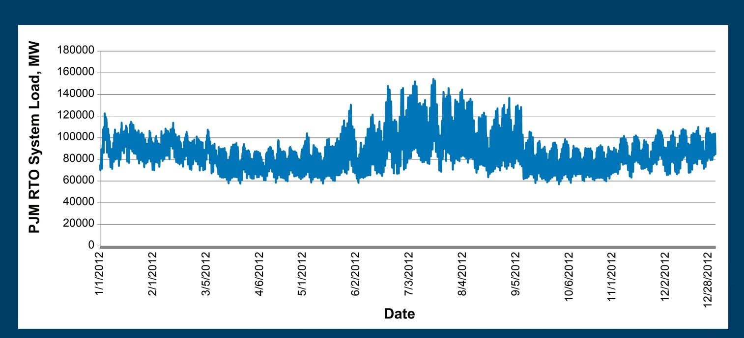
Electrical system load is directly related to the emission of CO<sub>2</sub>. This shows the variation of the system load for the PJM Interconnection Regional Transmission Organization in the eastern United States during 2012.
