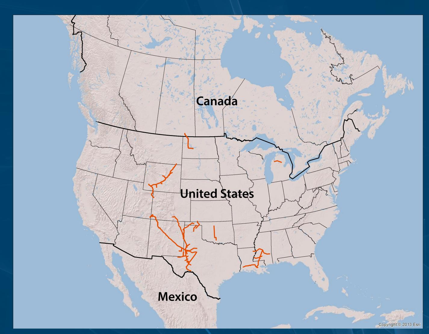
There are more than 6600 km (4100 mi) of  $CO_2$  pipelines in the United States. Additional pipelines are planned in Canada and the United States, but are not shown on this map.
