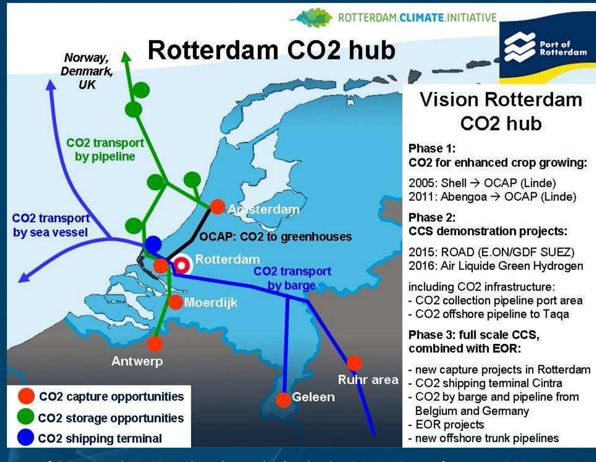
Map of the Rotterdam  $CO_2$  Hub in the Netherlands. The OCAP  $CO_2$  pipeline carries  $CO_2$  through a 97-km pipeline from a refinery to greenhouses to enhance plant growth.<sup>1</sup>
