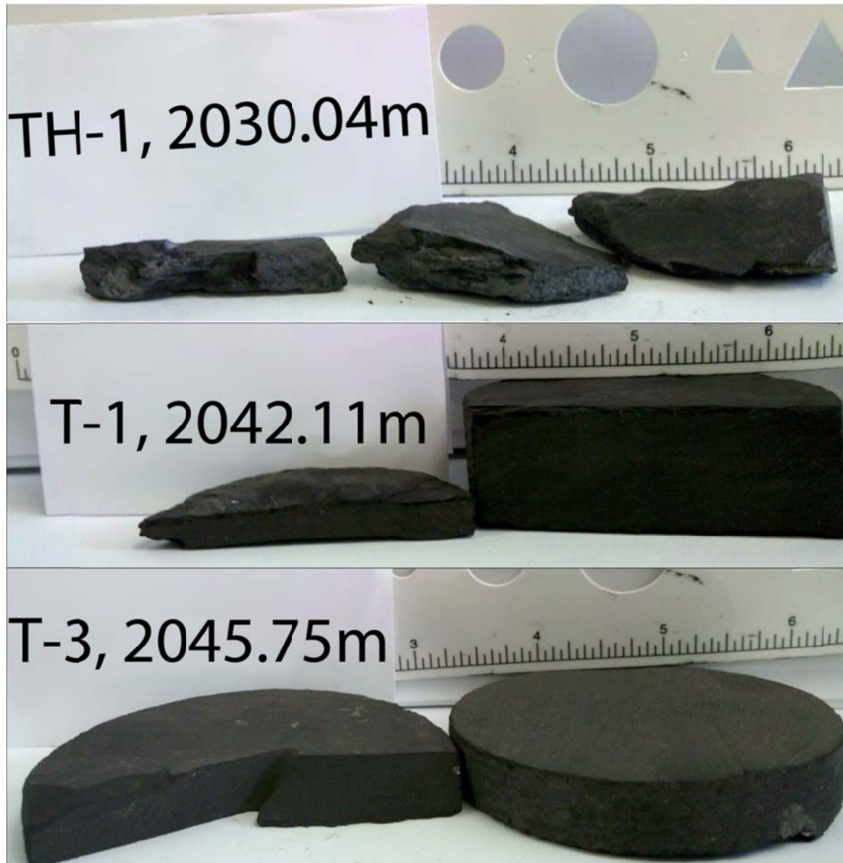
Figure 5. Photographs of Fort Nelson cap rock samples as received. These samples represent three cap rock intervals present in the Fort Nelson area.
