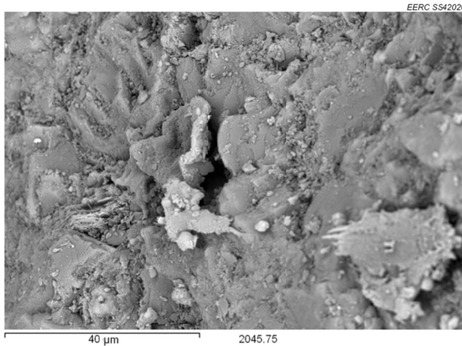
Figure C-20. SEM photomicrograph of T-3, fractured, 1500× magnification, showing mixed dolomite and clay matrix.
