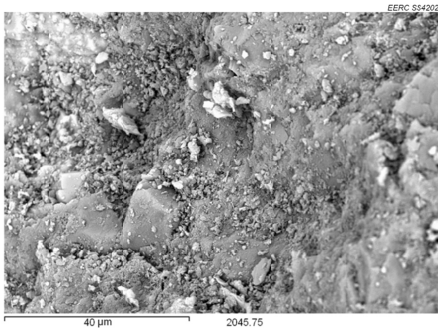
Figure C-21. SEM photomicrograph of T-3, fractured, 1500× magnification, showing dolomite and pyrite in illite clay.
