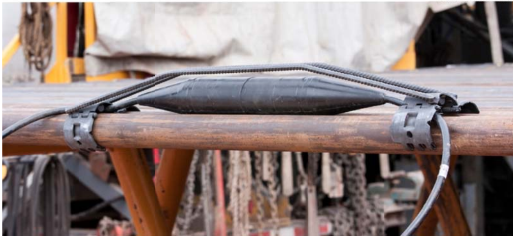
Figure 9. Geophone resting on 2 7 / 8 -in. tubing prior to downhole installation in 04-03 OW in the Bell Creek Field (April 2013).
