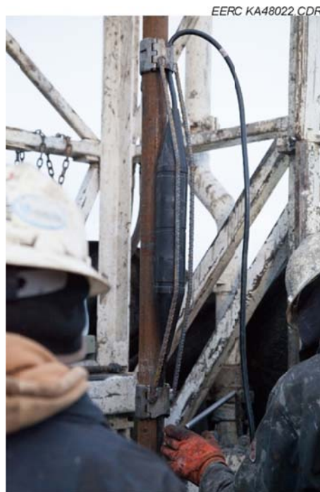
Figure 10. Rebar bracket protecting the geophone during downhole installation in 04-03 OW in the Bell Creek Field (April 2013).
