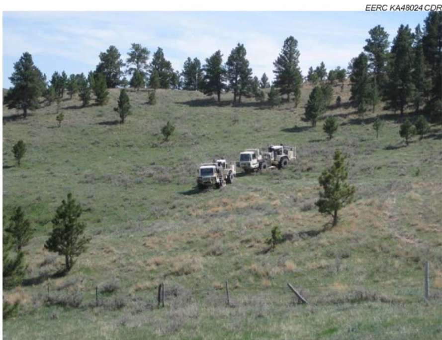
Figure 8. Two 60,000-pound Vibroseis units provide the source energy at a grid of nearly 1000 shot points surrounding two receiver wells. This survey provides a baseline before injection of CO 2 begins (May 2013).
