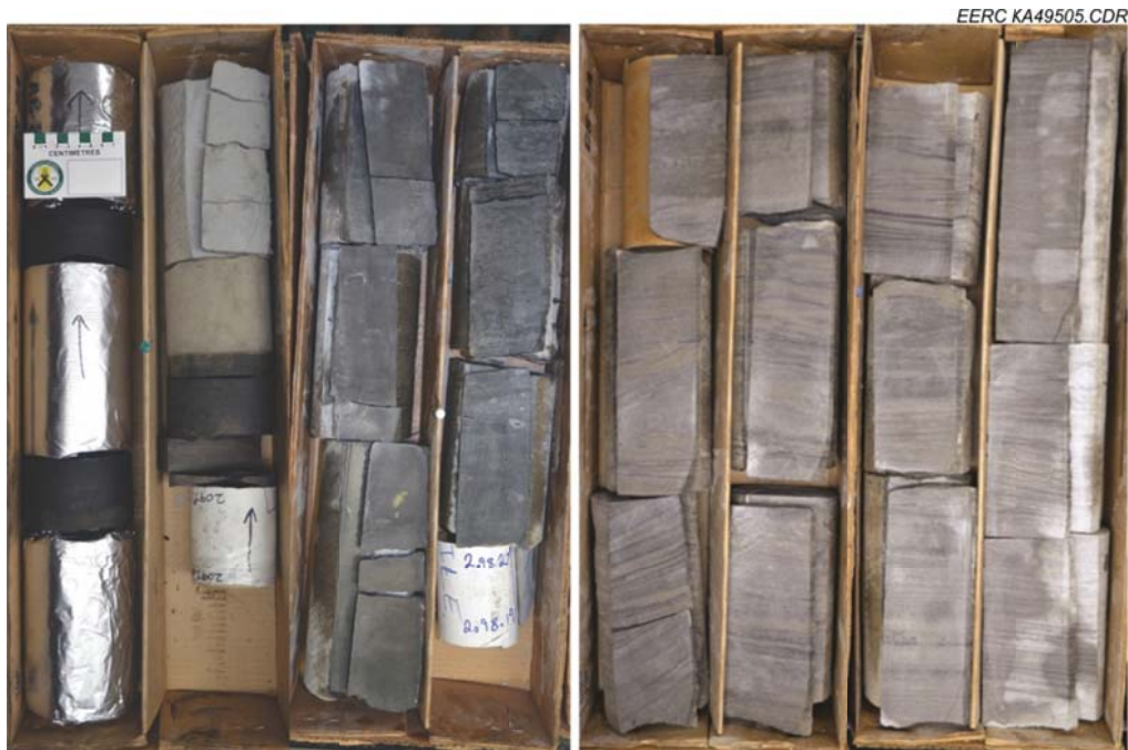
Figure 3. A continuous section of rock core from the Aquistore project well located near Estevan, Saskatchewan. The above figure provides an example of the upper shale interval (left) and middle laminated zones (right) of particular interest to regional characterization efforts.
