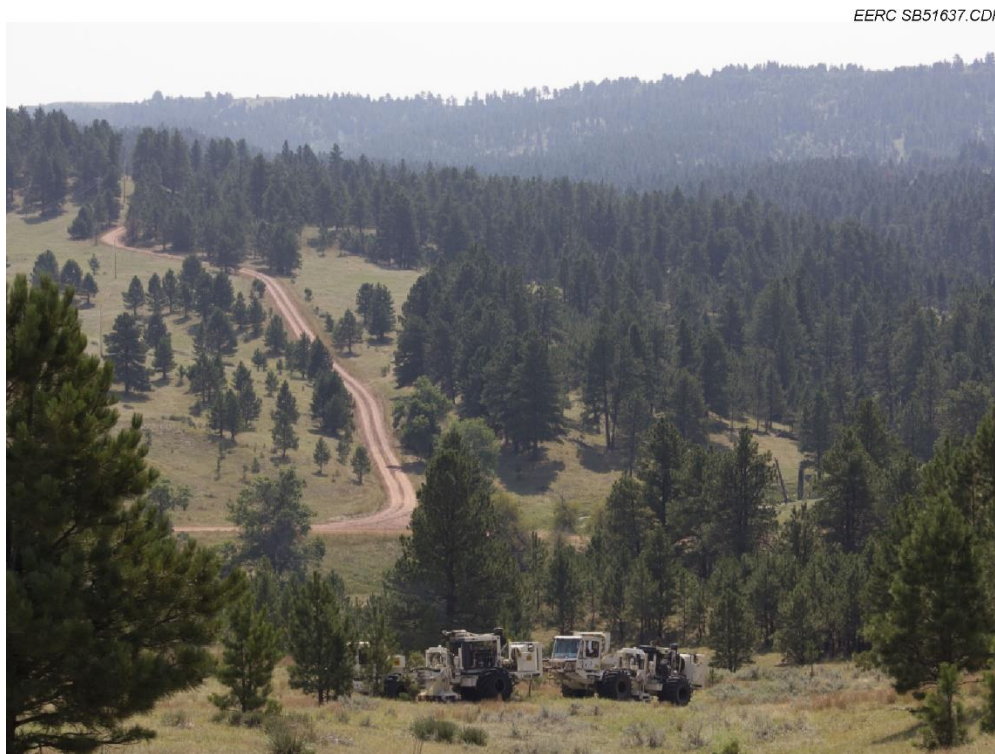
Figure 12. Vibrators working in the southern portion of the expanded baseline survey area.
