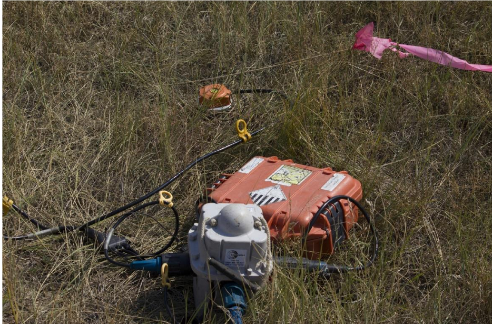
Figure 13. Nodal geophone assembly on station. From the top, a pin flag marking the surveyed receiver location, three-component geophone with leveling bubble, field battery, and Sercel Unite digital acquisition unit with GPS (global positioning system) antenna dome.
