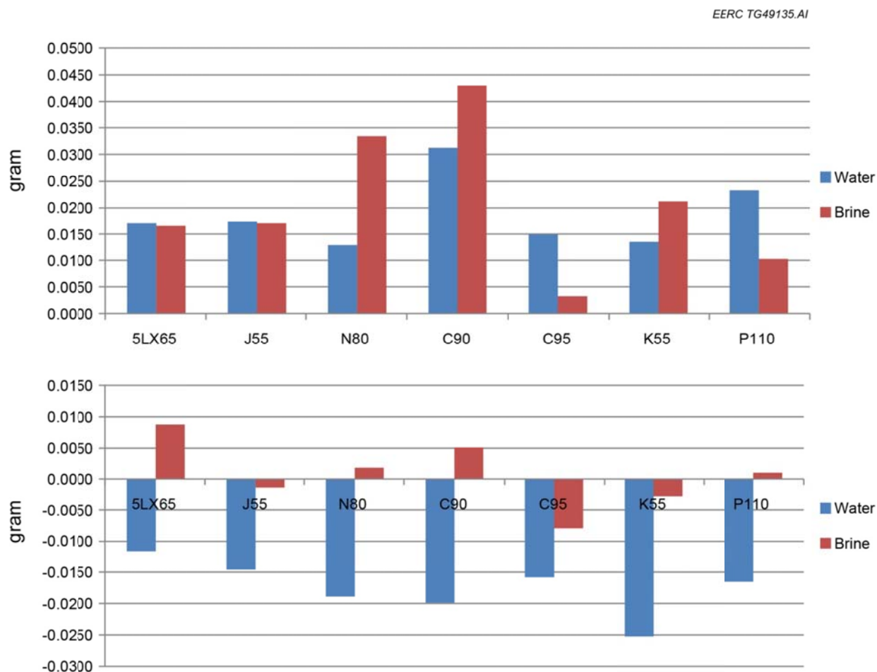
Figure 16. Mass differences between casing material coupons as measured before and after exposure to pure \text{CO}_2 (below) and \text{CO}_2 combined with \text{H}_2\text{S} (above) under both water (blue) and brine (red).
