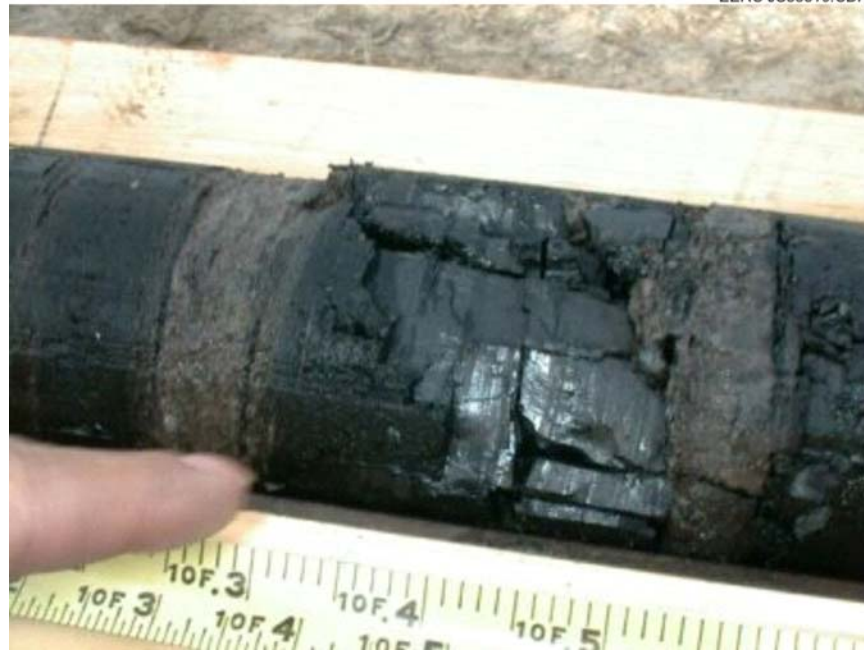
Figure 5-3. Burke County lignite coal core immediately after collection and prior to placement in canister for gas content analysis.
