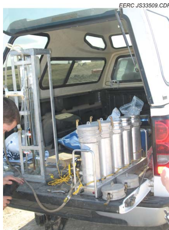
Figure 5-4. Canisters and field apparatus used to initiate gas desorption tests at the study site.
