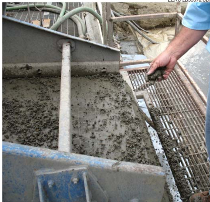
Figure 4-3. Shaker from which drill cuttings were collected.
