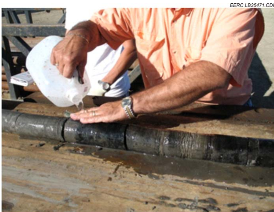
Figure 5-2. Preparing coal core for canister test.
