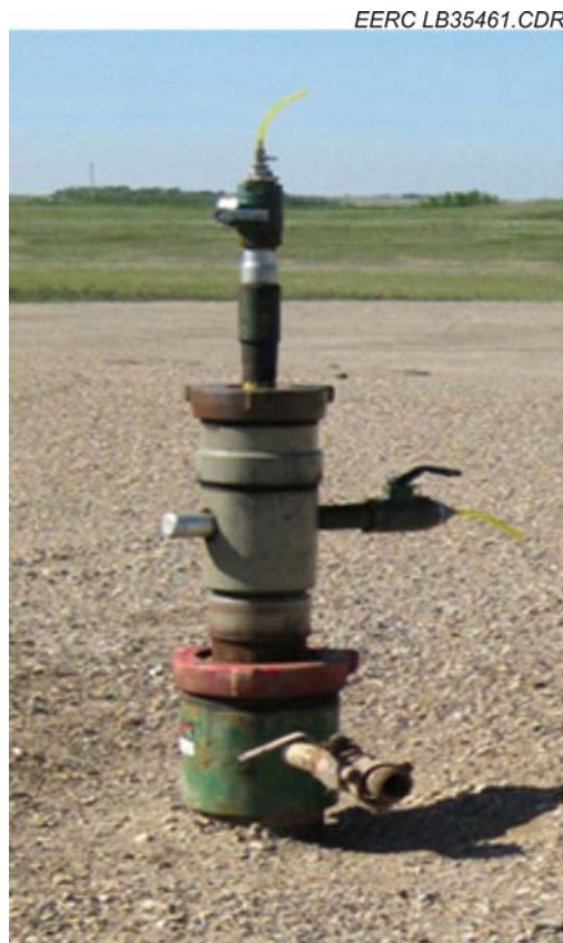
Figure 6-1. Pressure and gas access points.
