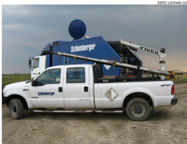
Figure 4-5. Photo of Schlumberger logging truck and sonde.
