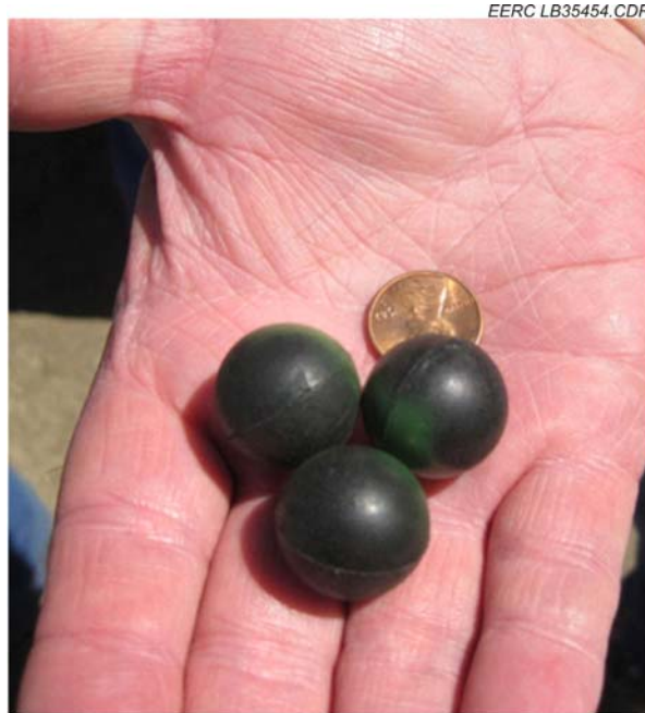
Figure 7-3. Perforation balls using during acid job.
