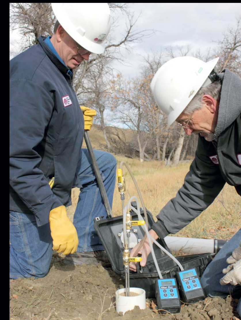
Soil gas sample collection at a fixed-location soil gas profile station
