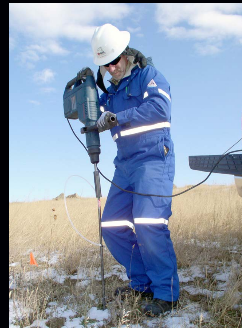
Soil gas probe sampling
