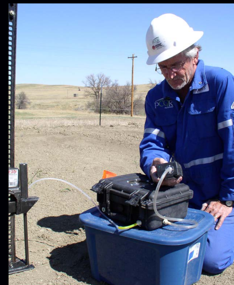
Handheld field meter analysis for soil gas survey
