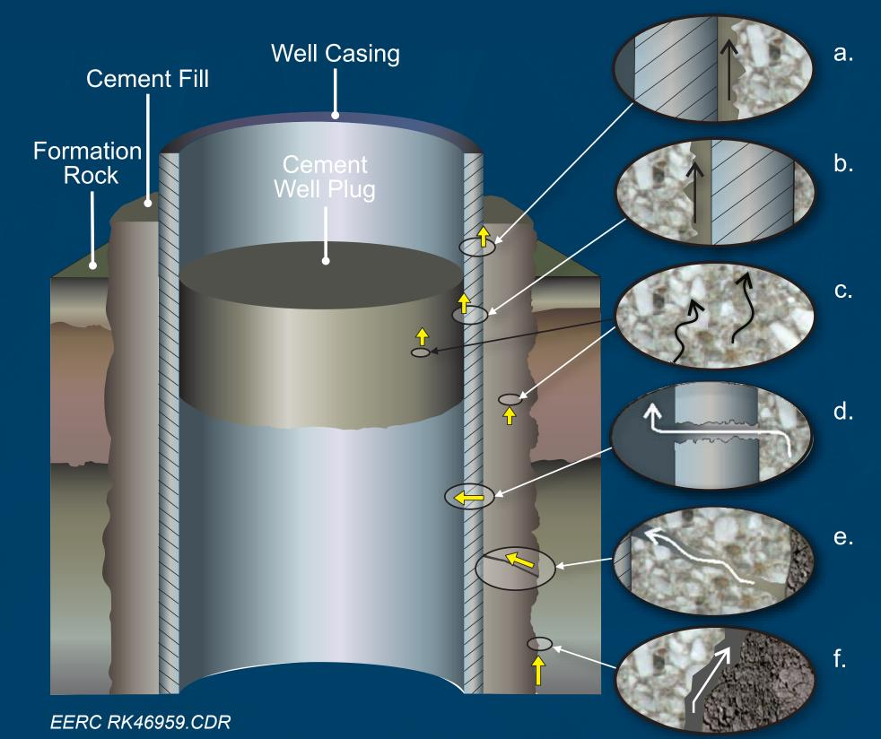
Conceptual illustration of the potential leakage pathways for CO, in a well along the casing-cement interface (a and b), within the cement (c), through the casing (d), through fractures (e), and along the cement-formation interface (f) (from Celia and others<sup>4</sup>).
