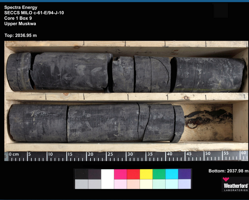
Core sample of the Muskwa formation collected from the exploratory well. The Muskwa Formation is a shale that will serve as a seal.
