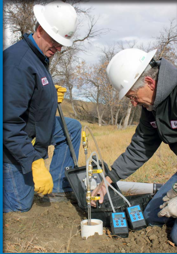
Soil gas sample collection at a semi-permanent soil gas profile station.
