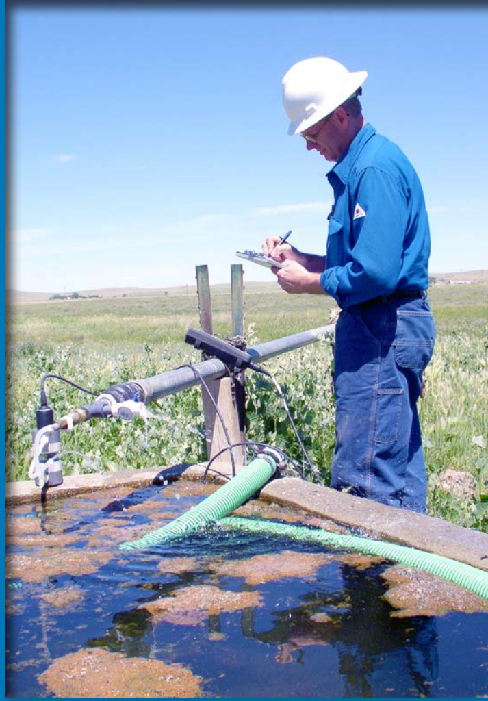
Groundwater sample collection at a stock well.
