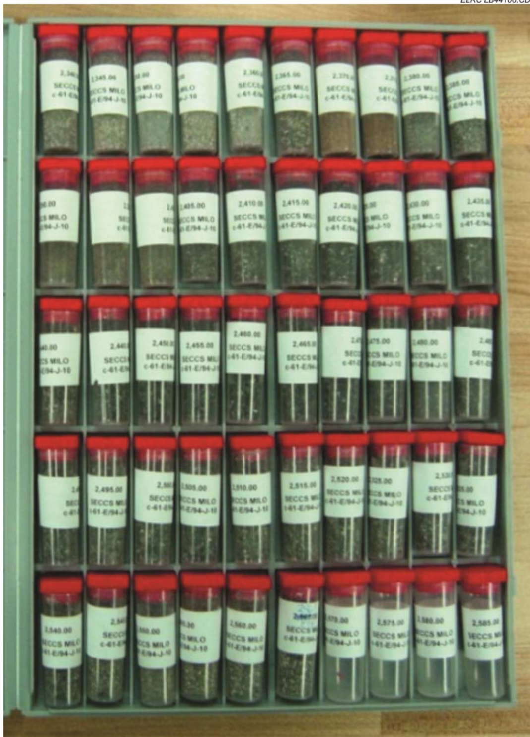
Figure 4. Example of as-received drill cuttings from Exploratory Well c-61-E.
