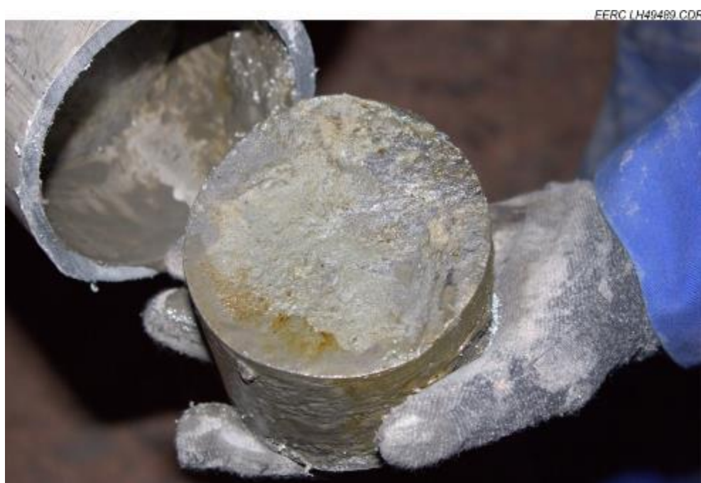
Figure 6. Example of core sample being extracted from the aluminum tubing used during the coring process.
