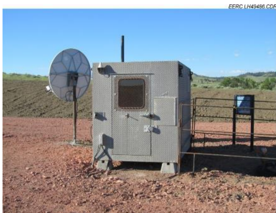
Figure 13. A small recording unit was placed on the surface at the 04-03 OW wellhead to continuously record passive seismic events and for use in the acquisition of 3-D VSPs.
